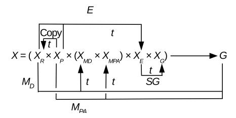
Fig. 9: Adding memories for evaluations of percepts  $(X_E)$  and for a current goal  $(X_G)$  to Fig. 7d. Connections to W have been elided for clarity.
